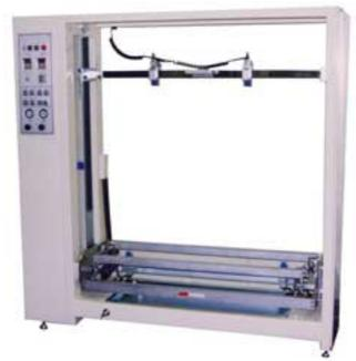
The most important factor of screen printing quality is technics of screen mask. By MEDIA MCM series which emulsion coating is automatically operated enable precise screen mask by standardization of uniform coating process. And it is simple to use.
