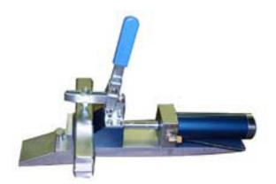
It is necessary for the correctness and beautiful image printing to make up the stencil which stretched more strong tension. By our original air cylinder, You can get more stronger and correctness tension.
